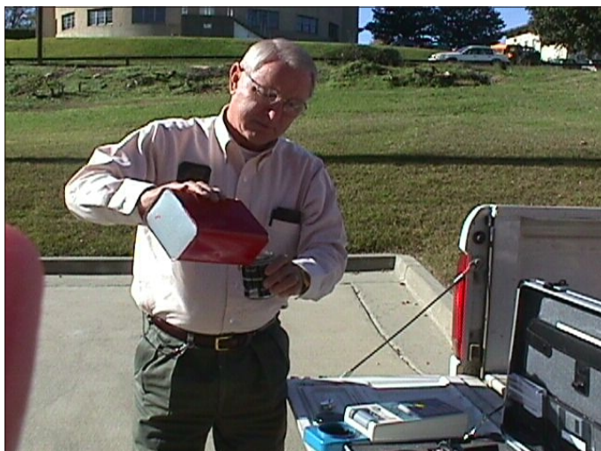
Field Supervisor Gerald Broom preparing an octane screening test using the Zeltex Octane Tester.
