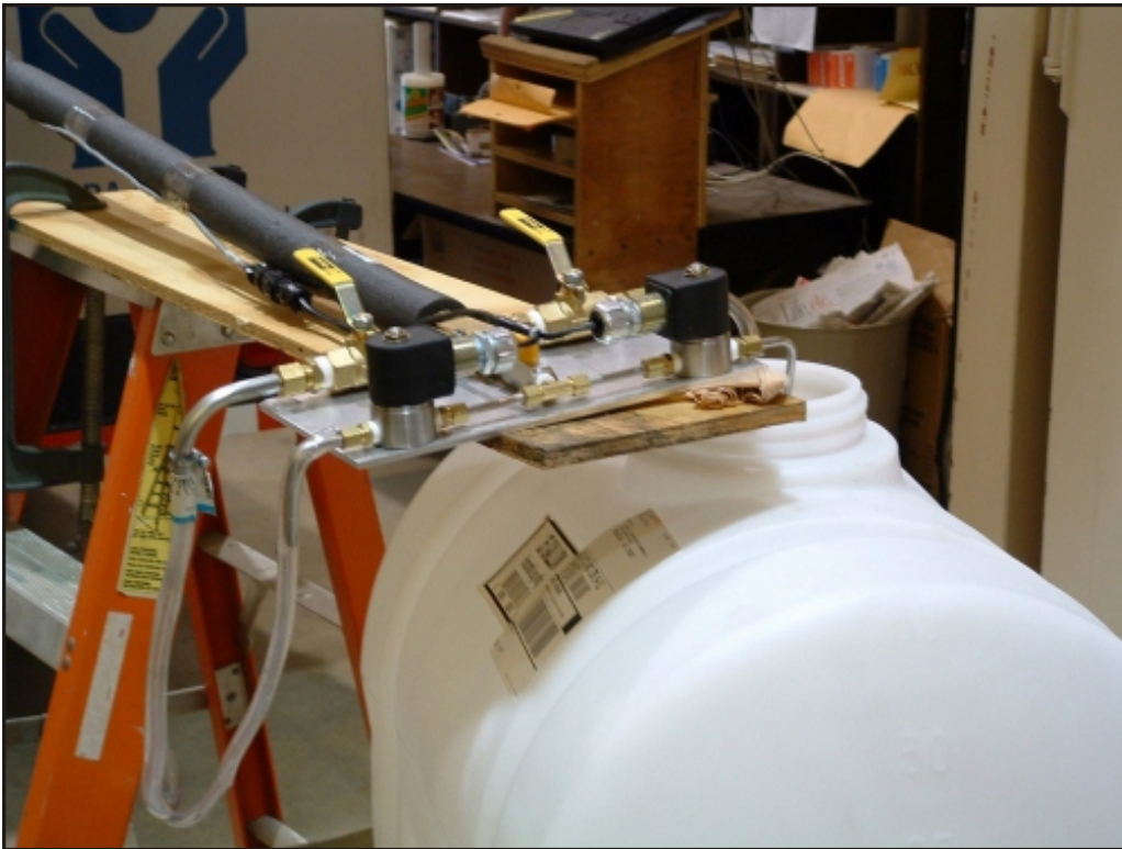
The calibration kit (solenoid controlled valves) needed to calibrate the provers.
