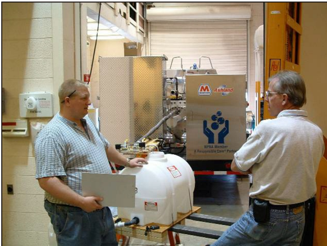
NC Metrologist Van Hyder discusses the prover calibration with Mike Honsberger of Marathon Ashland. The water from the calibrated section of the prover is weighed in the plastic tank.
