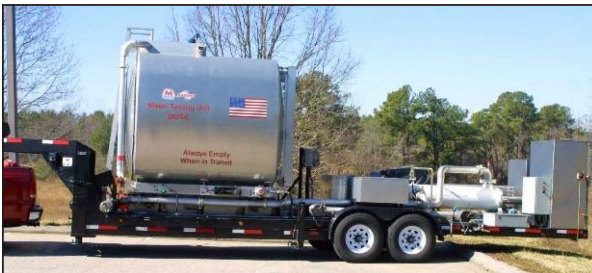
Marathon Ashland's first unit with a higher storage tank at the front of the trailer. The 20-gallon Calibron Syncrotrak SVP is the tube directly behind the axles.
