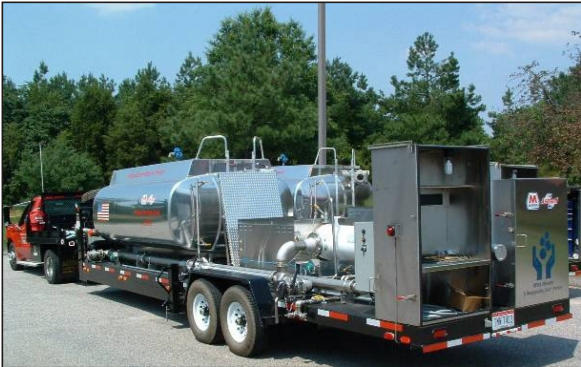
One of the Marathon Ashland SVP units in the back parking lot of the lab. The 20 gallon Calibron Syncrotrak SVP is the cylinder with a pipe flange just behind the trailer axles. The front section of the tank is a storage tank designed to eliminate back pressure problems experience when pumping directly back to storage.
