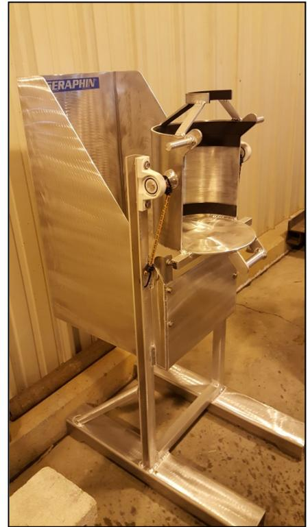
Testing Table/Sink for 5 gallon test measures
